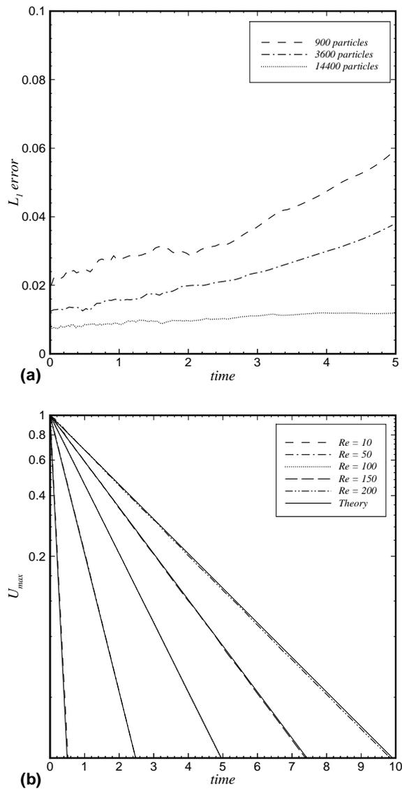
FIG. 2: Taylor-Green problem with different resolutions and Reynolds numbers: (a) history of  $L_1$  errors, (b) decay of the maximum velocities.
