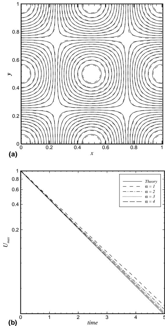
FIG. 1: Taylor-Green problem with  $Re = 100$ : (a) comparison between simulated vorticity profile (solid line) and analytical solution (dash line) at time  $t = 1$ , (b) simulated decay of the maximum velocity with different  $\alpha$ .
